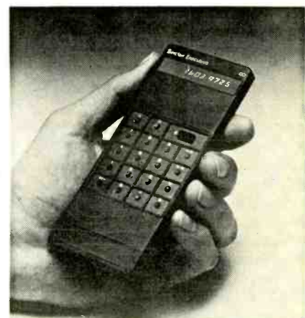
HAND-HELD ELECTRONIC CALCULATOR only \frac{1}{8} inch thick contains 7,000 transistors.
