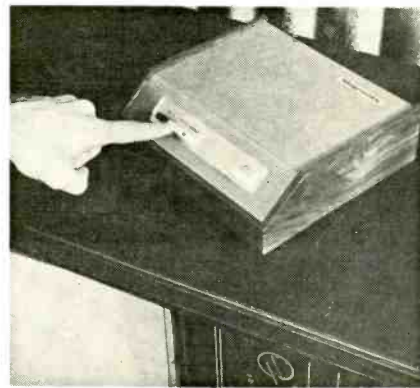
HOME TERMINAL CONTAINS CHANNEL switches and an "accept" button. Pushing either premium channel switch gives a preview of its program. The third switch is for ordinary CATV.
