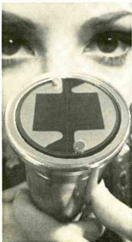
BIVICON CAMERA TUBE has two distinct pick-up surfaces—the dark rectangular areas.
