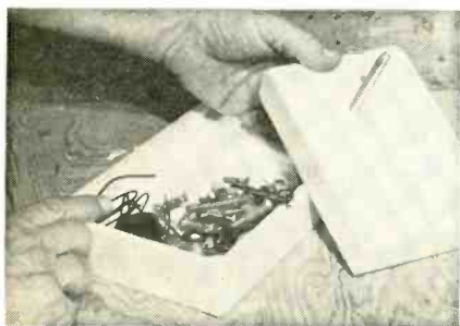
TWO HANDY BENCH AIDS made from foam plastic packing material used when shipping appliances and electronic devices.
